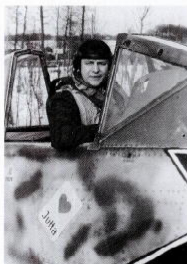
BELOW: At the end of 1943, Obstlt. Walter Oesau introduced a new emblem for Jagdgeschwader 1 consisting of a red winged '1' in a white diamond on a red disc. This Bf 109 G-6 'White 3', of 7./JG 1, carries the red JG 1 defence of the Reich band on its rear fuselage. Note also the DF loop and Erla canopy.
