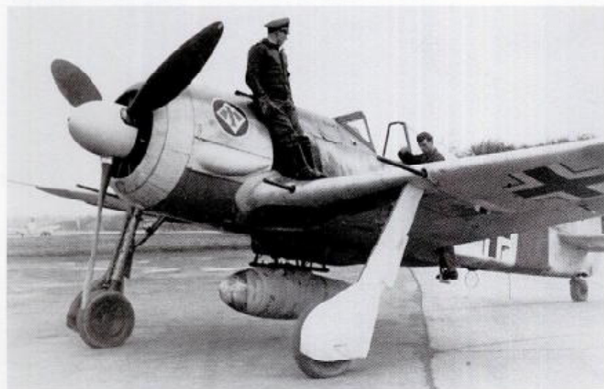
LEFT: Hptm. Alfred Grislawski, Staffelführer of I./JG 1, with his Fw 190 A-7 'White 9' at Dortmund in early 1944. Note that the 13 mm MG 131 machine guns mounted above the engine have been fitted with flash suppressors so that when flown on night operations the pilot's night vision was not impaired. Note also that the tip-mounted pitot tube on the starboard wing is more characteristic of the A-8 series, with which JG 1 would progressively re-equip from April 1944. Although the tone of the lower engine cowling panel matches that of the red fuselage band, it is thought that this is due to the type of film used and that the lower panel was yellow. This aircraft, W.Nr. 430965, was lost in combat with USAAF heavy bombers while being flown by Gefr. Alfred Martini of 2./JG 1 on 22 February 1944.
