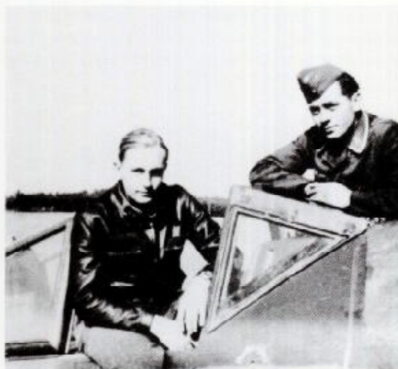
ABOVE LEFT, ABOVE AND ABOVE RIGHT: Three views of an Fw 190 A-8, WNr 170397, showing the armoured glass panels, or Panzerscheiben, similar to those fitted to the windscreen and canopy of Sturmstaffel 1's Fw 190 A-6s and A-7s to protect the pilots during their close range attacks against formations of USAAF four-engined bombers. The photograph above left and right shows the plate of 50 mm strengthened glass added to the windscreen, while the photographs centre and right show respectively the 30 mm armoured glass quarter panels fitted to the sides of the windscreen and the side panels added to the canopy.
