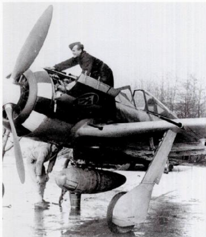
LEFT: While a member of the ground personnel opens the access panel to the BMW 801 D-2 engine of an Fw 190 A-7 of I./JG 1, another fills the drop tank mounted under the fuselage. Note the circular Panzer Ölkühler, or armoured oil cooler, on the front of the engine.
