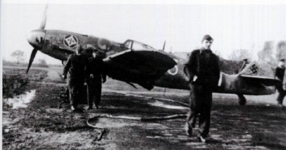
BELOW: At the end of 1943, Obstlt. Walter Oesau introduced a new emblem for Jagdgeschwader 1 consisting of a red winged '1' in a white diamond on a red disc. This Bf 109 G-6 'White 3', of 7./JG 1, carries the red JG 1 defence of the Reich band on its rear fuselage. Note also the DF loop and Erla canopy.
