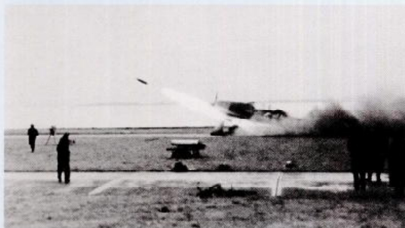
ABOVE: Fw 190A-5, W.Nr. 1372, 'White 4' of the weapons testing and evaluation unit, Erprobungskommando 25, was used to conduct firing trials with the 21 cm air-to-air mortar. Built by Focke-Wulf in Marienburg, it is believed the aircraft was with JG 1 before being transferred to Ekdo . 25. In this dramatic photograph, taken at Barth airfield, west of Stralsund on the north German coast in early 1944, a mortar is remotely fired from the aircraft for testing purposes and aimed across the waters of the Barther Bodden in the direction of Zingst.
