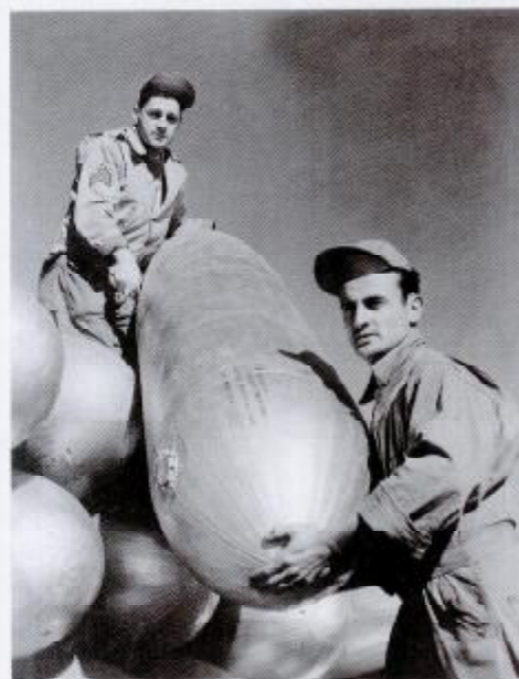
ABOVE: When the original US-made 200 gallon drop tank proved unsatisfactory due to leaks and fuel feed problems, a replacement was ordered but was not available for three months. To bridge the gap, a modified version of a resinated paper tank developed for the Hawker Hurricane was ordered and became available in July 1943 but not in quantities sufficient for large-scale operations. The early introduction of drop tanks allowed P-47s to fly to the Dutch/German border and surprised the Jagdwehhr, but when improved steel tanks became available, US fighters were able to fly deep within the Reich. This development represented a major threat to the Luftwaffe and many senior officers within the USAAF high command considered the drop tanks to be a weapon in themselves.
